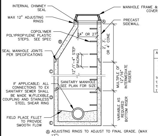
FRAME & COVER TO BE NEENAH R-1642A OR EQUAL. FRAMES WITH BOLT-DOWN LIDS SHALL BE NEENAH R-1916F
